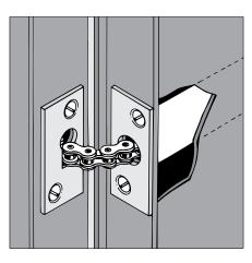
model) and insert the concealed jamb closer into the hole. If necessary the front plate can be embedded into the door leaf. It is fixed with two countersunk head screws. Fix the anchor plate exactly opposite and at the same height to the frame. Please make
