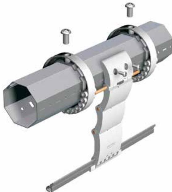
Upper automatic lock (latch lock) is used for roller shutter locking. It is installed together with locking rings. Each meter of a shaft is equipped with two locks. The lock is in operating position when the curtain is closed and pressed to the floor, and the slats are closed. Upper automatic lock acts as a locking device under the following conditions:
